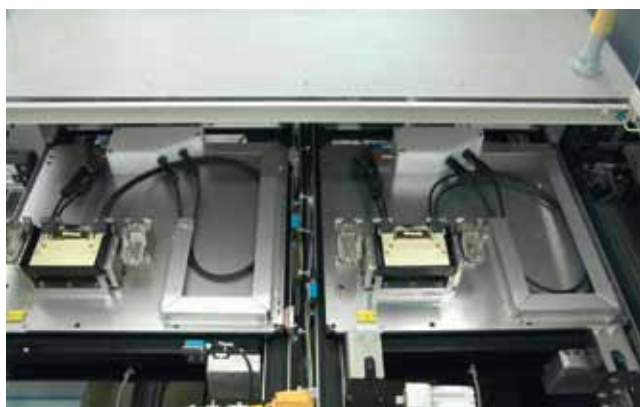
There are no off-the-shelf solutions for manufacturing power optimizers, so SolarEdge had to design its own bespoke automation system from scratch.
