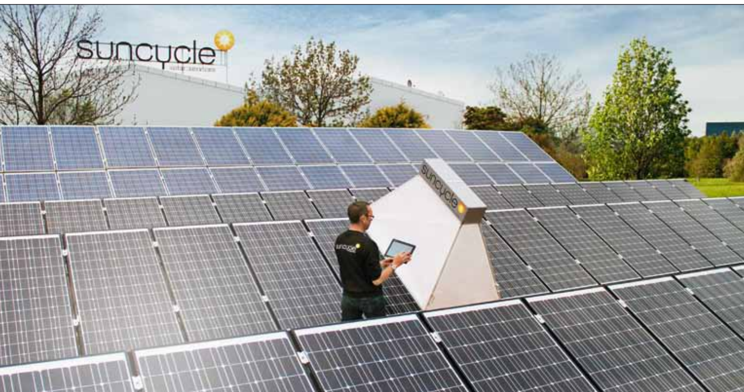
Suncycle detects PID directly in the array using electroluminescence testing.
